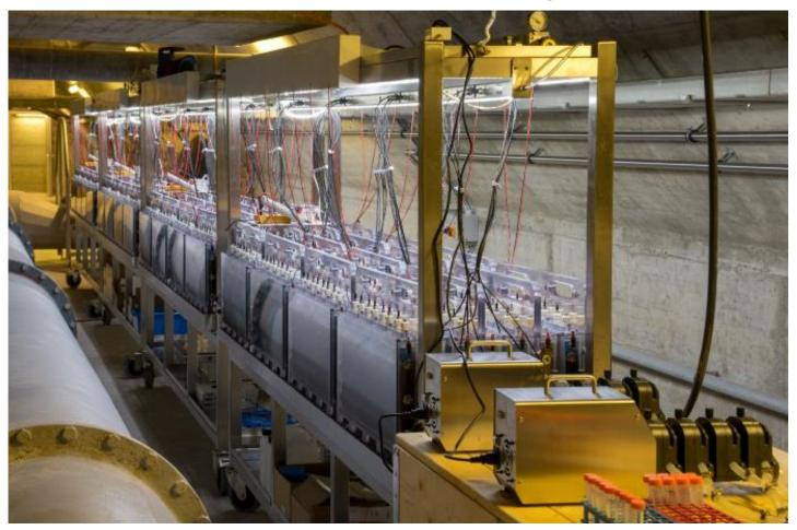
Safes and produces electricity from novel wastewater purification system. MFC scale up installation composed of 4 electrical independent carts for a total capacity of 1m<sup>3</sup> distributed within 64 microbial fuel cell units.
