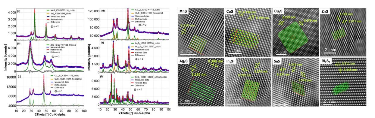
Lattice distances (from XRD and TEM) matches i.e. formation of phase pure metal sulfides; Highly crystalline particles
