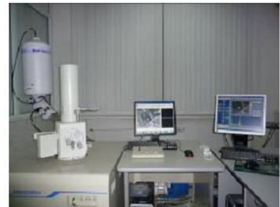
Scanning Electron Microscopy (SEM) by JSM-6390LV ("JEOL", Japan)
