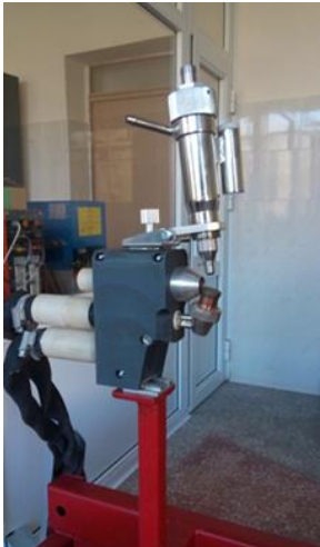
A pilot production site with an industrial complex for air-plasma metal cutting or microplasma spraying wire or powder coatings on the basis of an industrial robot Kawasaki RS-010LA (Kawasaki Robotics, Japan)
