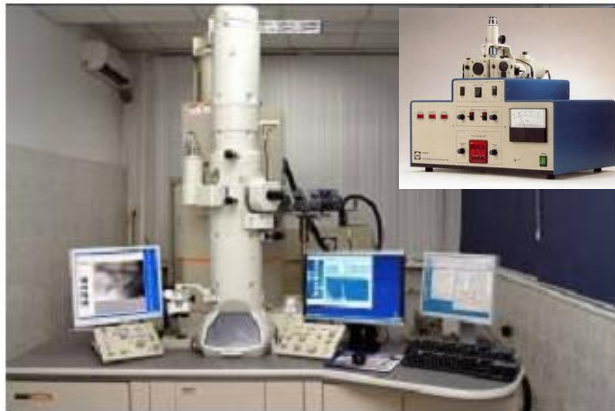
Transmission Electron Microscopy (TEM) by JEM-2100 ("JEOL", Japan) Precision Ion Polishing System M-691 ("Gatan", USA)
