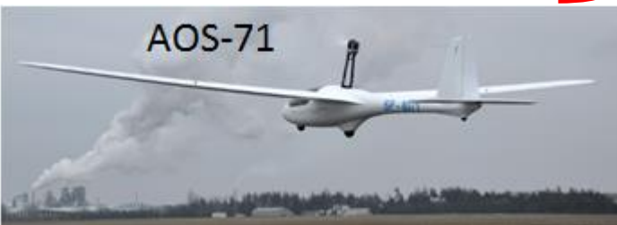
Electric motor-glider with lithium-polymer batteries
